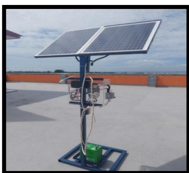
Gambar 6. Solar panel type Polycrystalline 2 x 50 WP, input daya 100 watt, output 220 volt / 1000 watt
