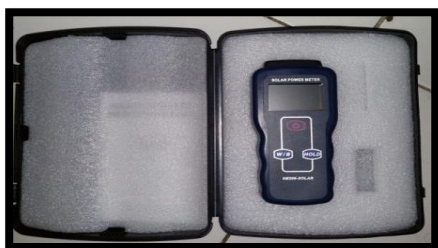
Gambar 4. Solar Power Meter type sun light tester intensity radiation SM-206
