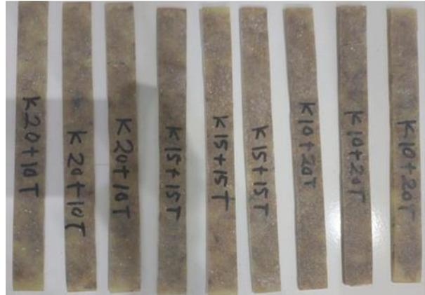
Gambar 6. Spesimen Uji Tarik ASTM D3039
