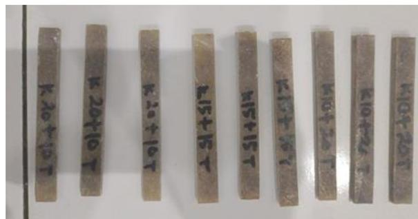
Gambar 7. Spesimen Uji Bending ASTM D7264
