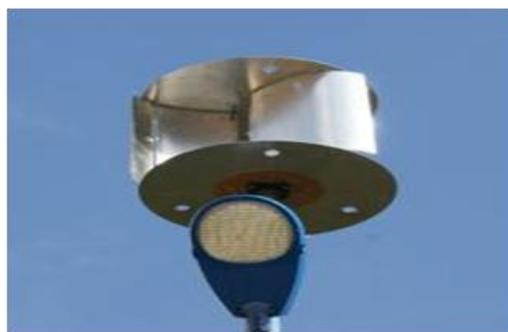
Gambar 4. Turbin Angin Tipe Savonius
