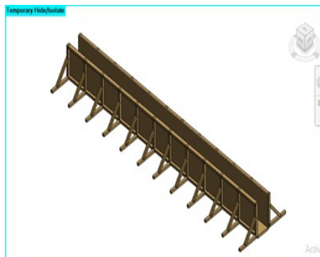
Gambar 6. Modelling bekisting balok
