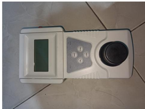
Gambar 4. *Turbidimeter Nephelometer* Jenis SGZ-200BS.
