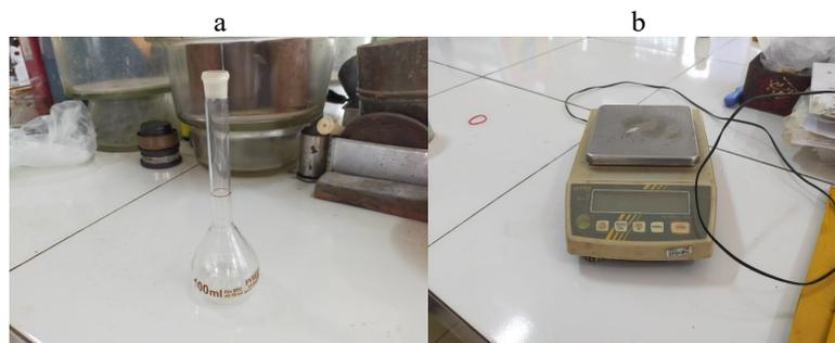
Gambar 5. (a) Piknometer 100 ml. (b) Neraca digital.
