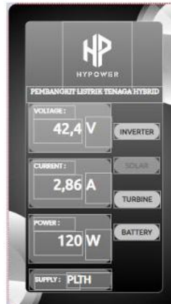
Gambar 4. Desain Tampilan Monitoring Solar Cell
