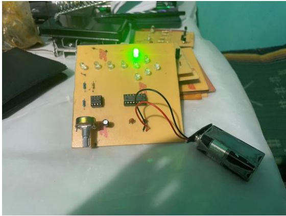
Fig. 3. Printed Circuit Board (PCB) Assembly of The Running LED Circuit During Practicum Activities
