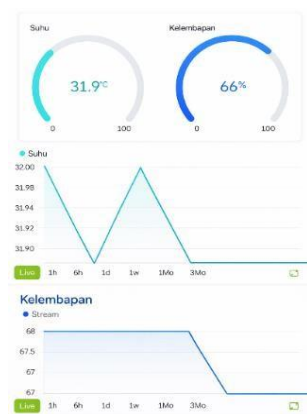
Figure 4. Monitoring Interface on Blynk Application
