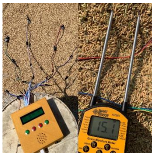
Gambar 13. Capacitive Soil Moisture Sensor dan Grain Moisture Meter AR991
