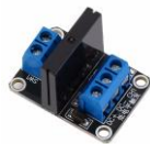
Gambar 3.6 Modul Relay 1 Chanel [26]
