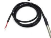
Gambar 3.3 Sensor Suhu DS18B20 [20]
