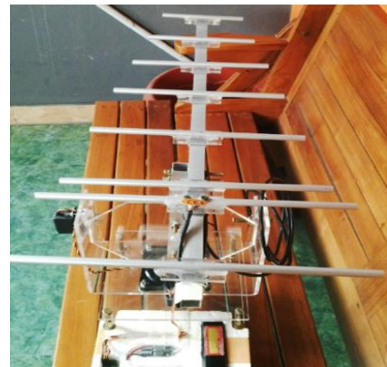
Gambar 3. Antena Yagi \frac{1}{2} \lambda 8 Elemen
