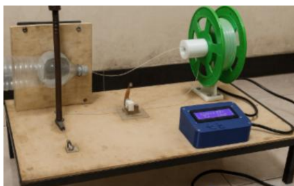
Figure 8. Plastic Bottle Recycling Machine into 3D Printer Filament
