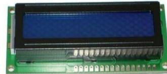
Gambar 3 *Liquid Cristal Display* ( LCD)
