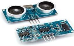
Gambar 2. 8 Sensor Ultrasonik
