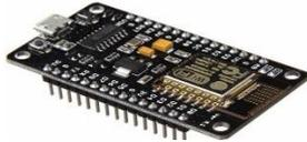
Gambar 1 *NodeMcu* ESP8266
