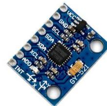
Gambar 2. Sensor MPU 6050.
