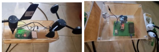
(a) Transceiver (b) Receiver Gambar 8. Pengujian modul lora
