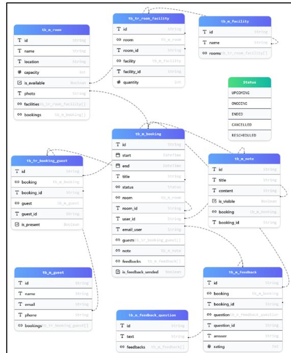
Gambar 8 Skema ORM Prisma (UML)
