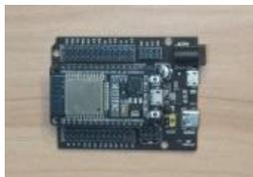
Gambar 1. NodeMCU ESP32
