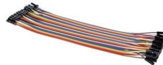
Gambar 11 *Kabel Jumper*
