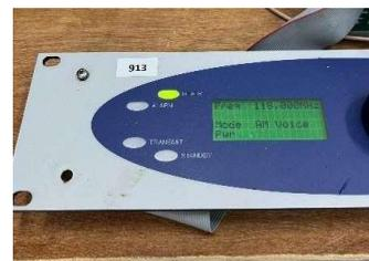
Gambar 12 Indikator alarm normal
