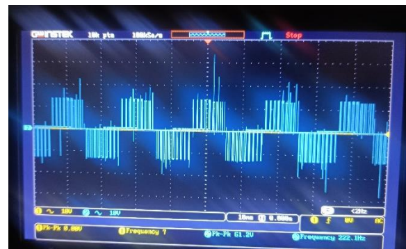
Gambar 10. Hasil tegangan line-line
