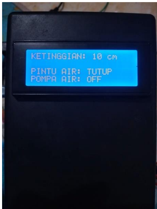
Gambar 6. Sistem Monitoring LCD16x2
