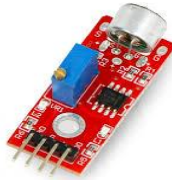
Gambar 2. Sensor Suara LM393 Electret Microphone
