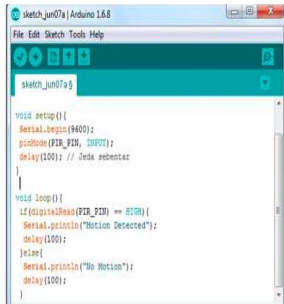
Figure 12. Program pengujian modul sensor PIR
