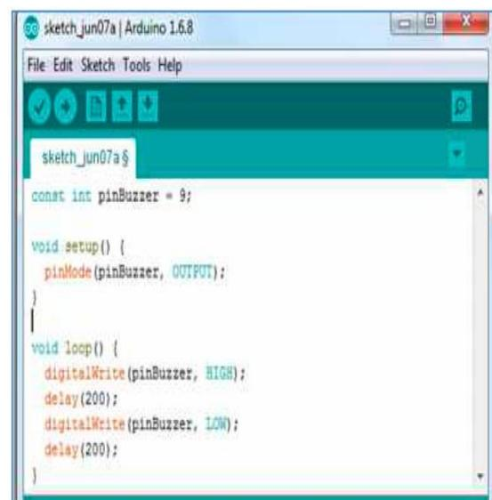
Figure 17. Program pengujian modul buzzer
