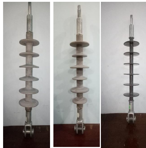
(a) (b) Gambar 1, Isolator uji (a). Isolator resin epoksi different shed dan same shed (b). Isolator silicone rubber (buatan pabrik).
