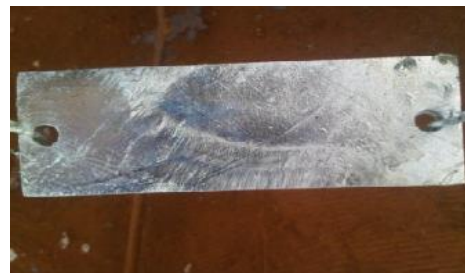
Gambar 4. Hasil proses pelapisan hot dip galvanizing
