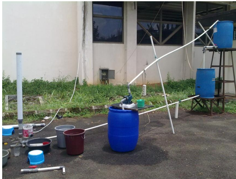
Gambar 2. Sistem instalasi model pengujian hydraulic ram pump .
