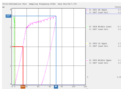
Gambar 2. Grafik hasil uji tarik current design
