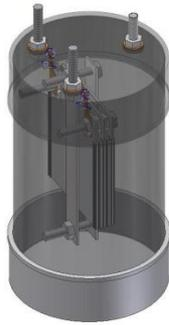
Gambar 1. *Hydrogen generator*
