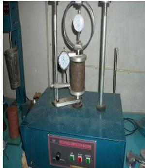
Gambar 2. Uji CBR Laboratorium
