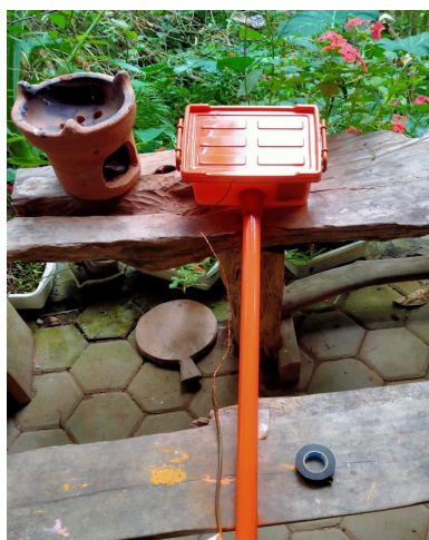
Gambar 3. Alat ukur sedimen tersuspensi berbasis Turbidity Sensor (NTU-18).
