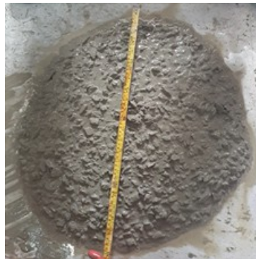
Gambar 3. Pengukuran Diameter Slump Flow
