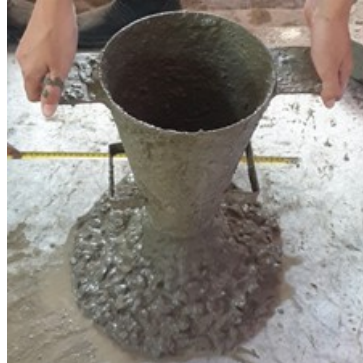
Gambar 2. Pengujian Slump Flow Test
