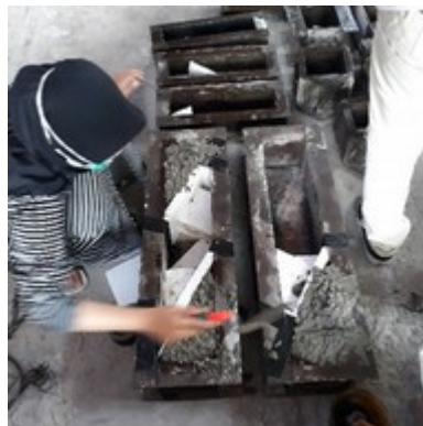
Gambar 3. Proses pengecoran beton lama ( substrate ).
