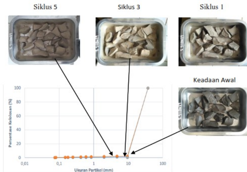
Gambar 11. Hasil uji Accelerated Slaking Test batuan Lemong
